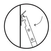
Insert the hangers into the wall rail. Position the hangers so the Hook & Loop aligns with the rear of the panels.
